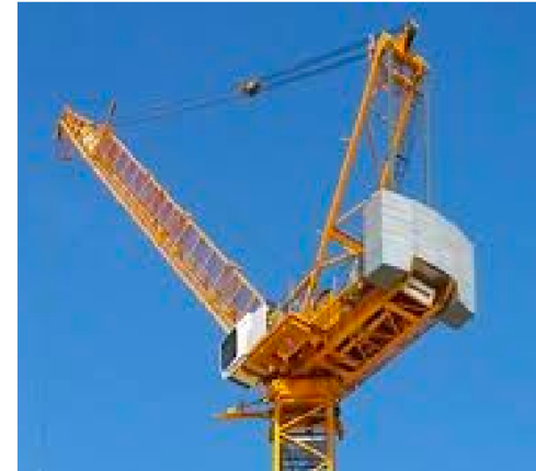
Luffing crane (Image: Cranemag.com)
